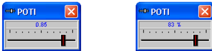
Control window of the slider with absolute resp. relative digital display
