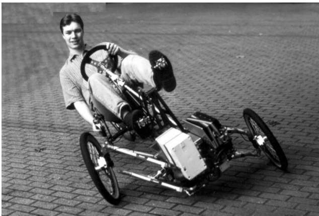
Fig. 1. Virage2000, human powered and hydraulic tilting, UaSB in 1999
