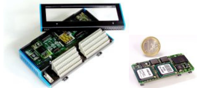
Fig. 11. Sorcus DIP5 subminiatur processor system
